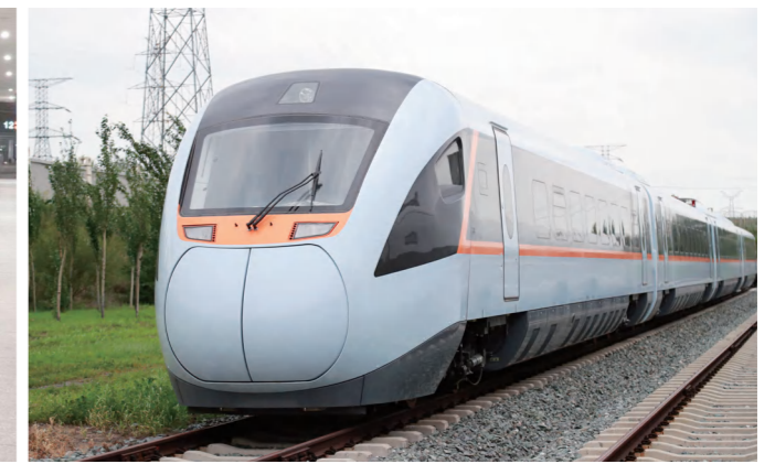
CJ5E型混合动力城际动车组 CJ5E Hybrid Power Intercity EMU
