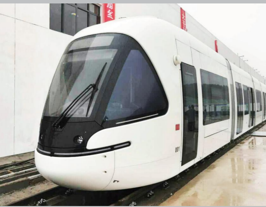
无网超能100%低地板有轨电车 Catenary-Free Super Capacity 100% Low Floor Tram
