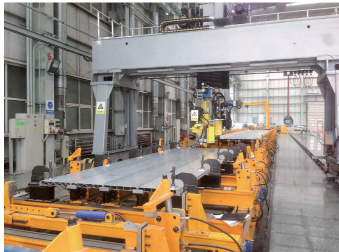
铝合金搅拌摩擦焊制造技术平台 Friction Stir Welding Manufacturing Platform of Aluminum Alloys
